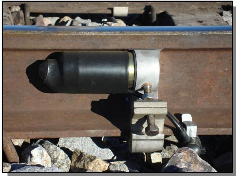
Receivers measure the pulse intervals to identify the direction of the specific Transmitter station. For this purpose, Receivers are also individually set to
